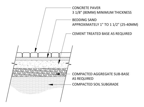
NOTE: PROVIDE DRAINAGE FOR BEDDING SAND
